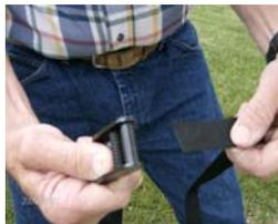
Long strap being placed through the bottom side of cam buckle the proper way.
