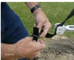
Place bottom long strap through bottom of short strap through cam buckle and pull through.
