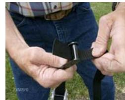
Long strap being pushed through the bottom side of cam buckle so teeth can grip the strap.
